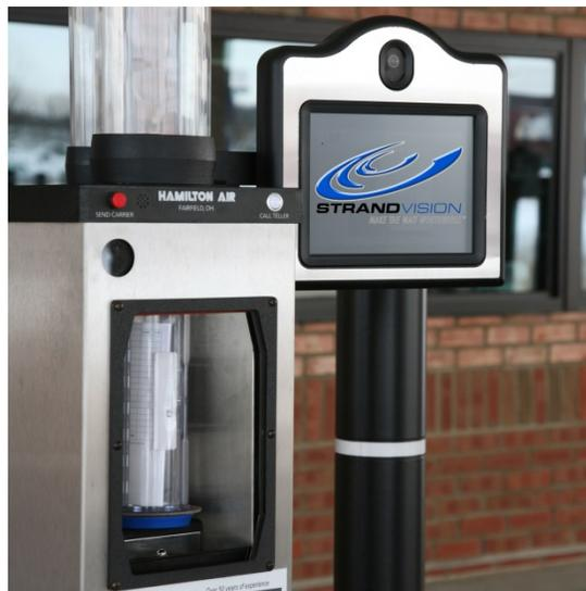
A dedicated digital media player, located in the data room, is directly integrated into the Hamilton Air drive-up kiosk equipped with an audio and two-way LCD video console using a standard RF converter. The system screen shows the teller whenever he/she activates the audio/video channel, and displays the digital signage content pages while the transaction is being completed and when the drive-up is idle between transactions. “The digital
